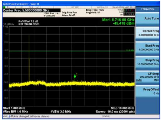
Test Plots (GFSK) - 1 GHz - 10 GHz (RBW:1 MHz, VBW: 3 MHz) Spurious Emission (High-CH)
