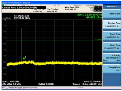
Test Plots (8DPSK) - 1 GHz - 10 GHz (RBW:1 MHz, VBW: 3 MHz) Spurious Emission (Mid-CH)
