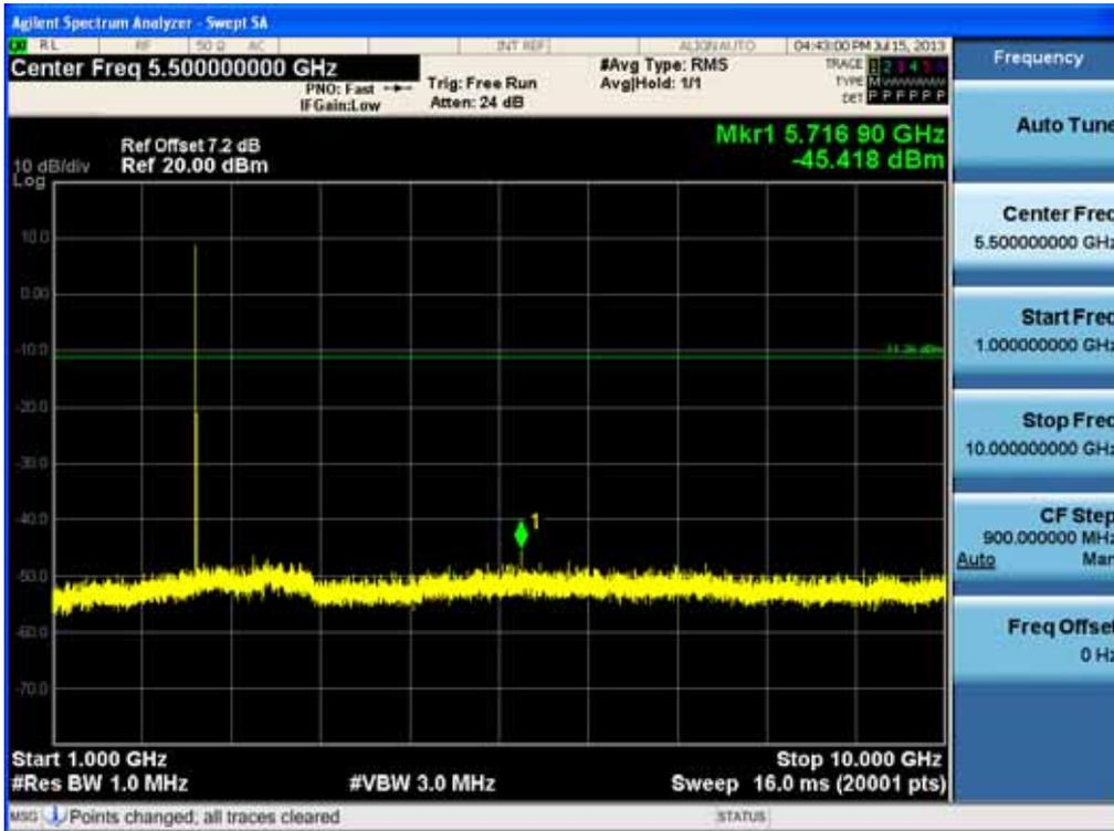
Test Plots (GFSK) - 1 GHz - 10 GHz (RBW:1 MHz, VBW: 3 MHz)
