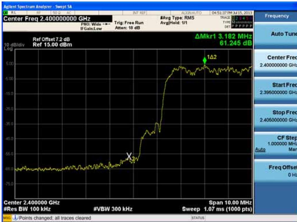
Test Plots with hopping (8DPSK)
