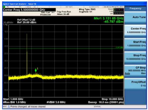
Test Plots ( $\pi$ /4DQPSK) - 1 GHz - 10 GHz (RBW:1 MHz, VBW: 3 MHz) Spurious Emission (High-CH)
