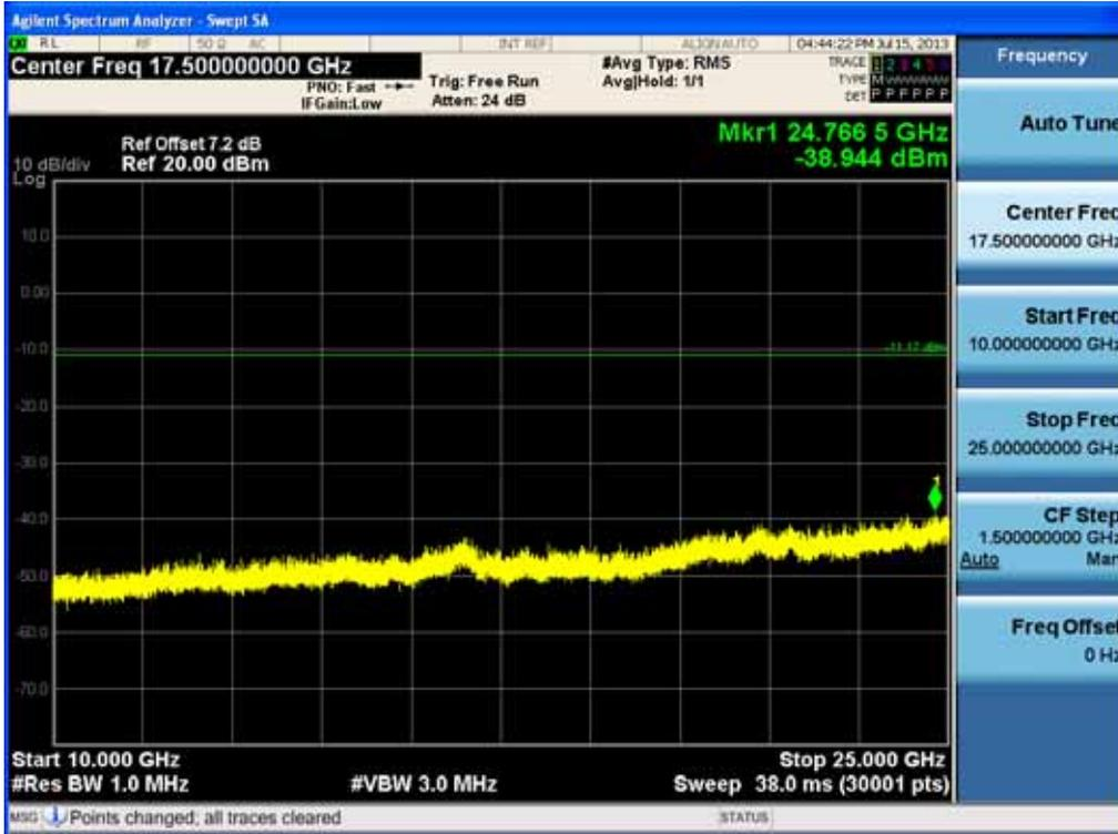
Test Plots (8DPSK) - 10 GHz - 25 GHz (RBW:1 MHz, VBW: 3 MHz)
