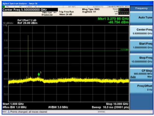
Test Plots ( $\pi$ /4DQPSK) - 1 GHz - 10 GHz (RBW:1 MHz, VBW: 3 MHz) Spurious Emission (Low-CH)
