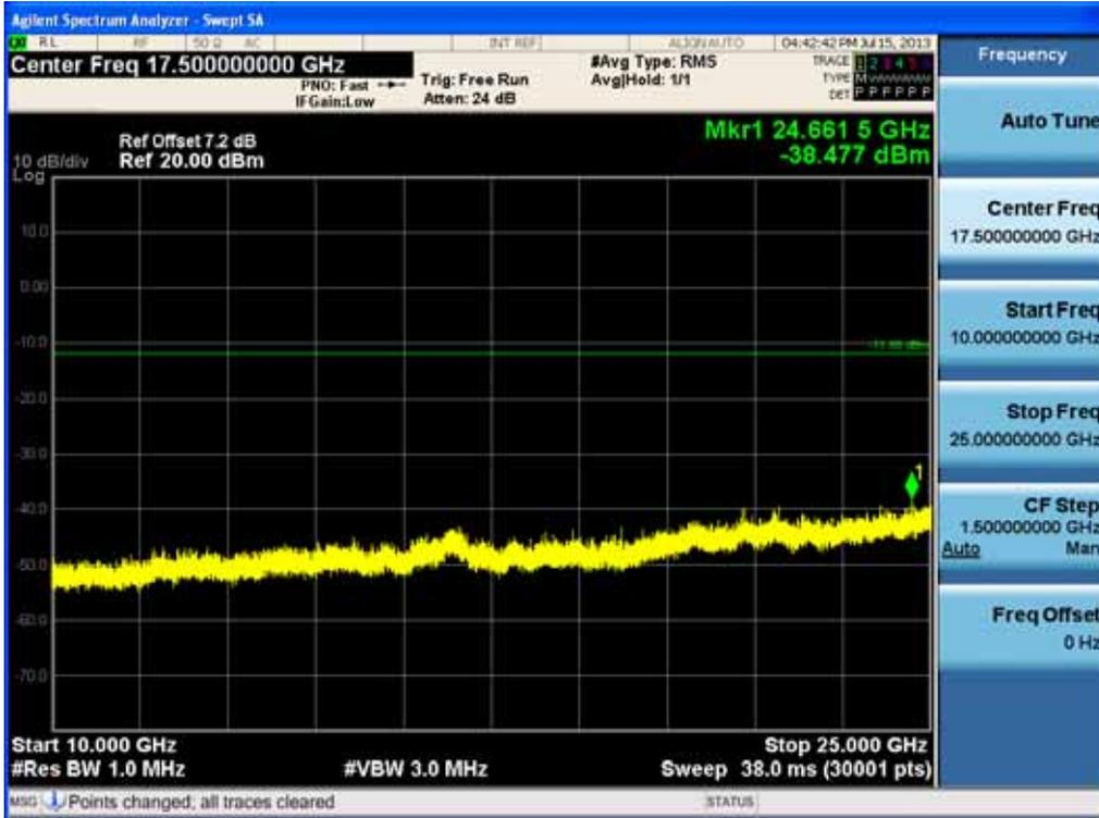
Test Plots (GFSK) - 10 GHz - 25 GHz (RBW:1 MHz, VBW: 3 MHz)
