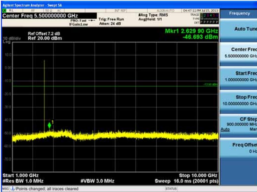
Test Plots (8DPSK) - 1 GHz - 10 GHz (RBW:1 MHz, VBW: 3 MHz)
