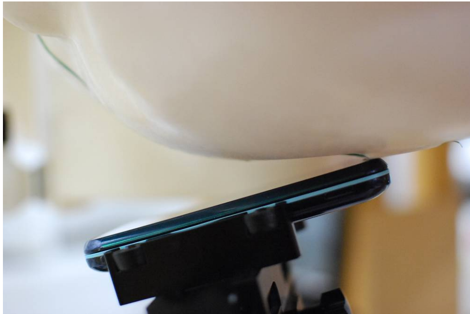
SAR Test Setup Photo 4: Left Tilt
