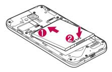
4 Align the battery cover over the battery compartment (1) and press it down until it clicks into place (2).
