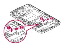
3 Insert the battery into place by aligning the gold contacts on the phone and the battery (1) and pressing it down until it clicks into place (2).
