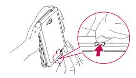
2 Push down and slide the SIM card into its slots as shown in the figure. Make sure the gold contact area on the card is facing downwards.
