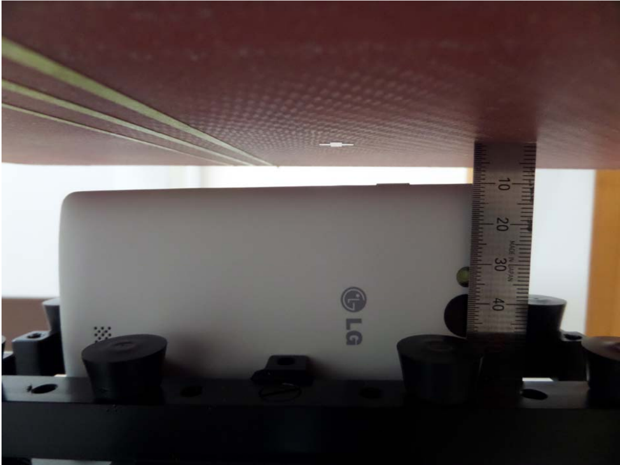
[Distance of 1.0 cm from the EUT]
