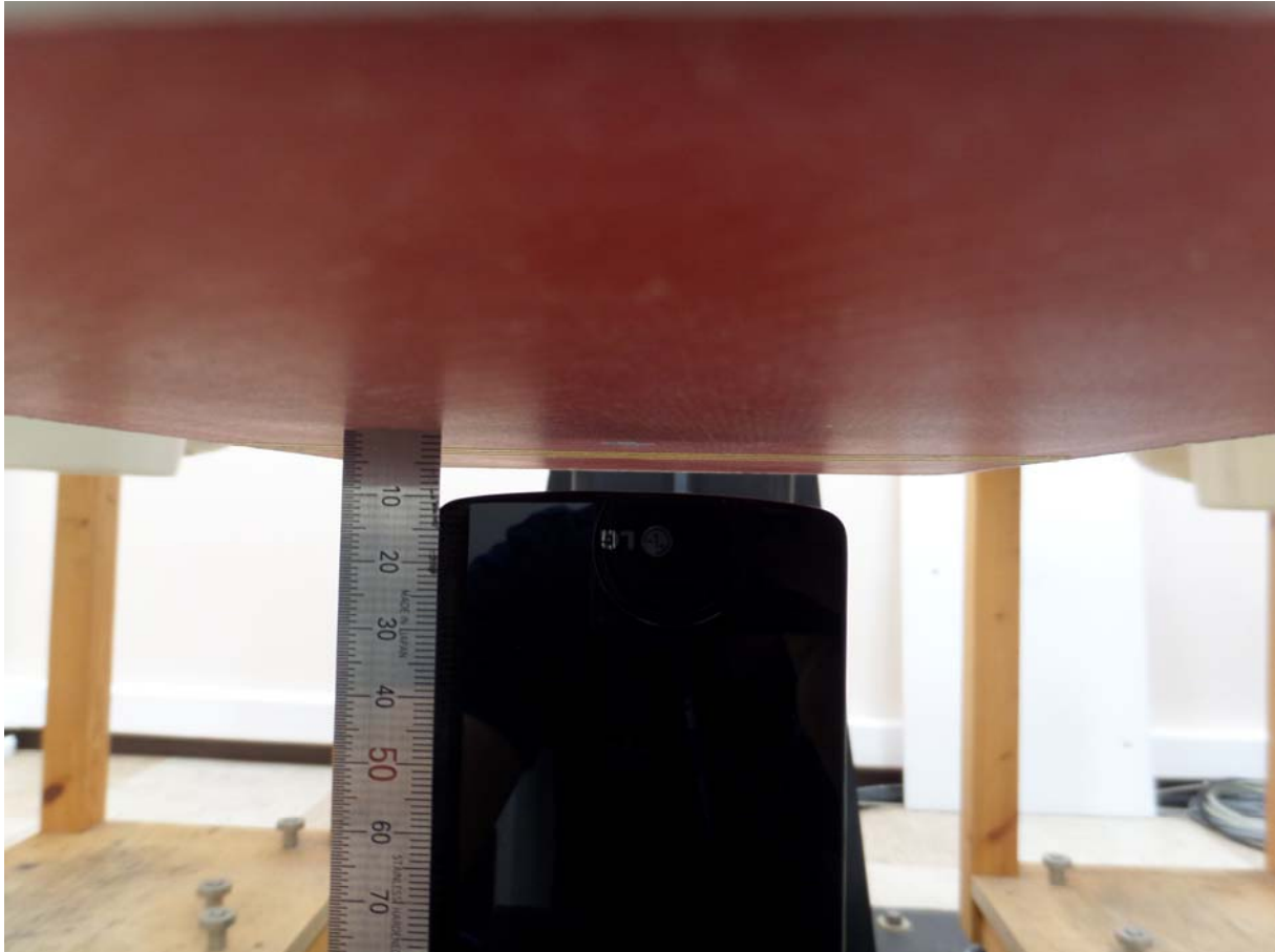
[Distance of 1.0 cm from the EUT]
