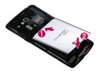
4 Align the battery cover over the battery compartment (1) and press it down until it clicks into place (2).
