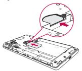
3 Insert the battery into place by aligning the gold contacts on the phone and the battery (1) and pressing it down until it clicks into place (2).
