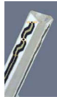
Figure 3.3 Probe Thick-Film Technique
