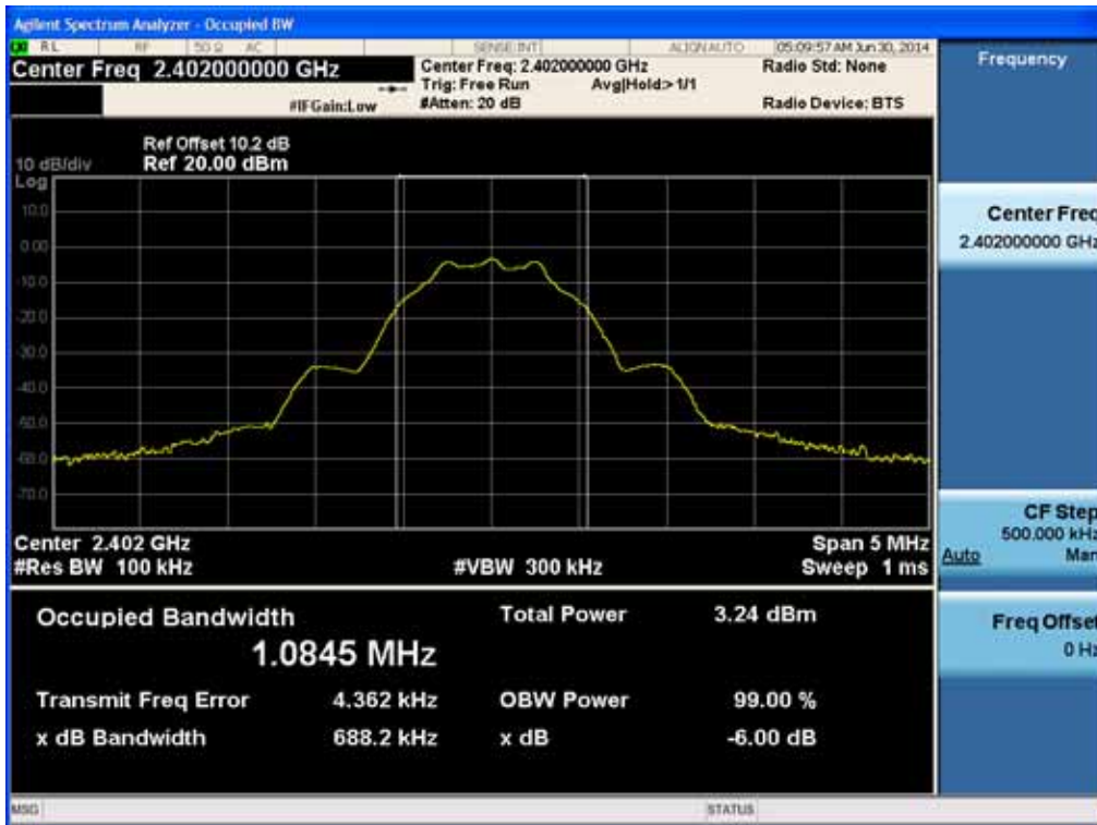
6dB Bandwidth plot (Low-CH 0)
