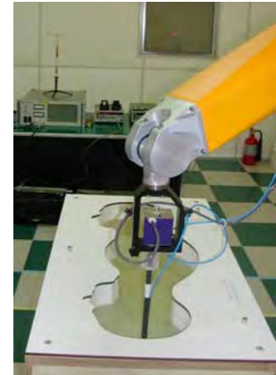
Figure 5. Photograph of the probe and the Phantom
