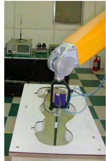
Figure 3. Photograph of the probe and the Phantom
