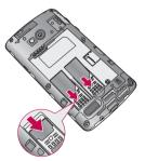
3 Insert the battery into place by aligning the gold contacts on the phone and the battery (1) and pressing it down until it clicks into place (2).
