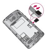
**NOTE:** Use only compatible memory cards with your phone. Using incompatible memory cards may damage the card and data stored on the card, as well as the phone.
