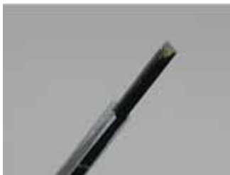
Figure 6. EX3DV4 E-field Probe
