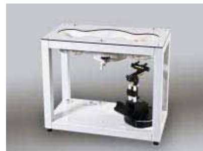
Figure 3.6 SAM Twin Phantom
