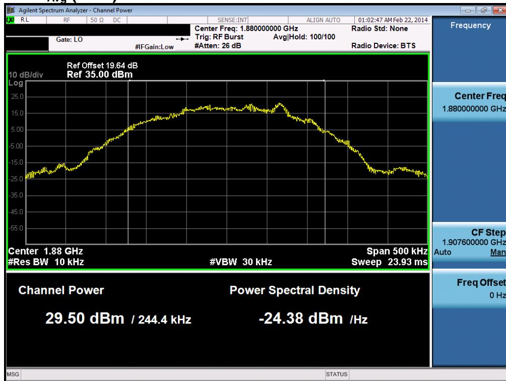
$$\text{PAPR (dB)} = P_{PK} (\text{dBm}) - P_{Avg} (\text{dBm}) = 29.634 \text{ dBm} - 29.500 \text{ dBm} = 0.134 \text{ dB}$$
