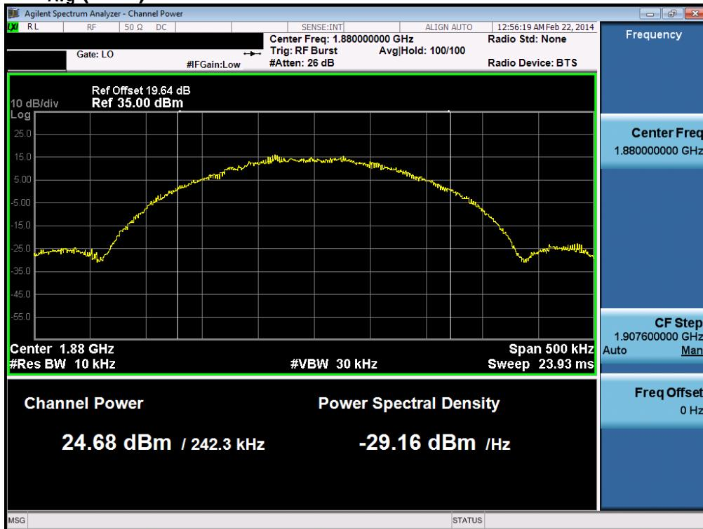
$$\text{PAPR (dB)} = \text{P}_{\text{pk}} (\text{dBm}) - \text{P}_{\text{Avg}} (\text{dBm}) = 29.14 \text{ dBm} - 24.68 \text{ dBm} = 4.46 \text{ dB}$$
