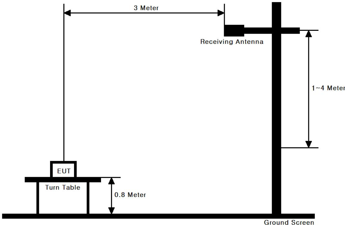
These measurements were performed at 3 & 10m test site. The equipment under test is placed on a wooden turntable 0.8-meters above the ground plane and 3-meters from the receive antenna. The receive antenna height and turntable rotations were adjusted for the highest reading on the receive spectrum analyzer.
