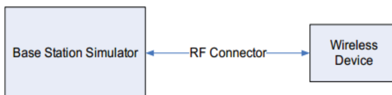
Figure 10.2 Power Measurement Setup
