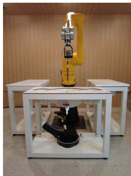
Figure 2.2 DASY5 Test System
