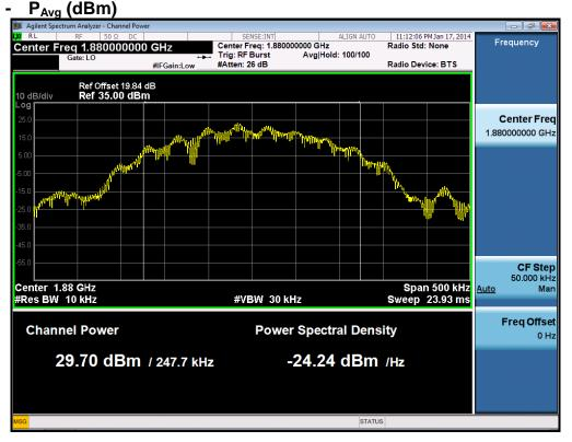
PAPR (dB) =  $P_{Pk}$  (dBm) -  $P_{Avg}$  (dBm) = 29.950 dBm - 29.700 dBm = 0.250 dB
