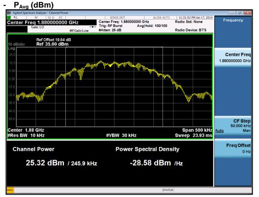
PAPR (dB) =  $P_{Pk}$  (dBm) -  $P_{Avg}$  (dBm) = 30.015 dBm - 25.320 dBm = 4.695 dB
