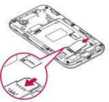
Insert the battery into place by aligning the gold contacts on the phone and the battery (1) and pressing it down until it clicks into place (2).
