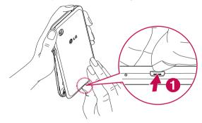
2 Slide the SIM card into its slot as shown in the figure. Make sure the gold contact area on the card is facing downwards.
