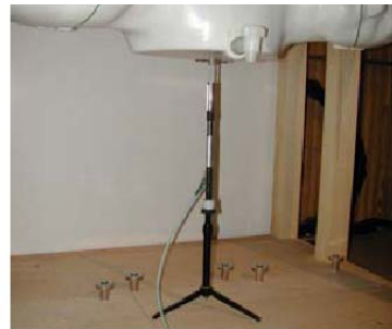
Figure 11.1 Dipole Verification Test Setup Diagram & Photo
