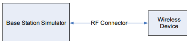
Figure 10.1 Power Measurement Setup
