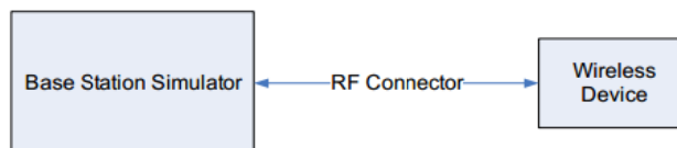
Figure 10.1 Power Measurement Setup
