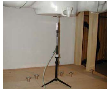
Figure 11.1 Dipole Verification Test Setup Diagram & Photo
