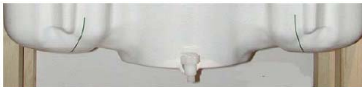
Figure 3.7 Sam Twin Phantom shell
