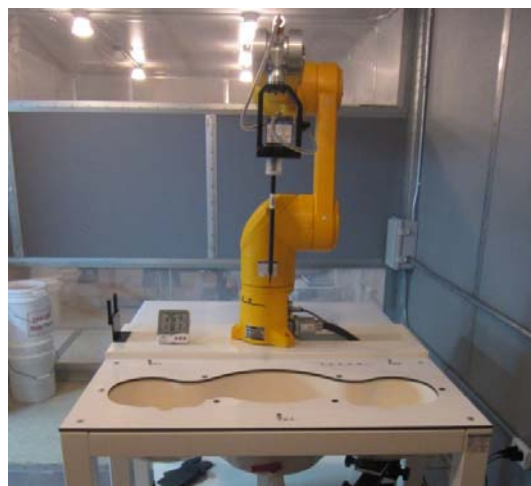
Figure 2.2 DASY5 Test System
