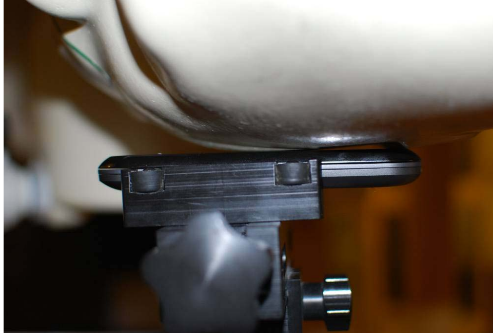
SAR Test Setup Photo 3 – Left Touch
