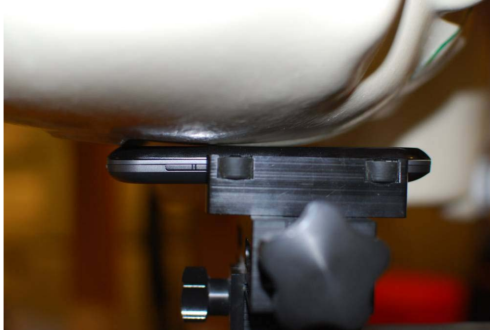
SAR Test Setup Photo 1 – Right Touch
