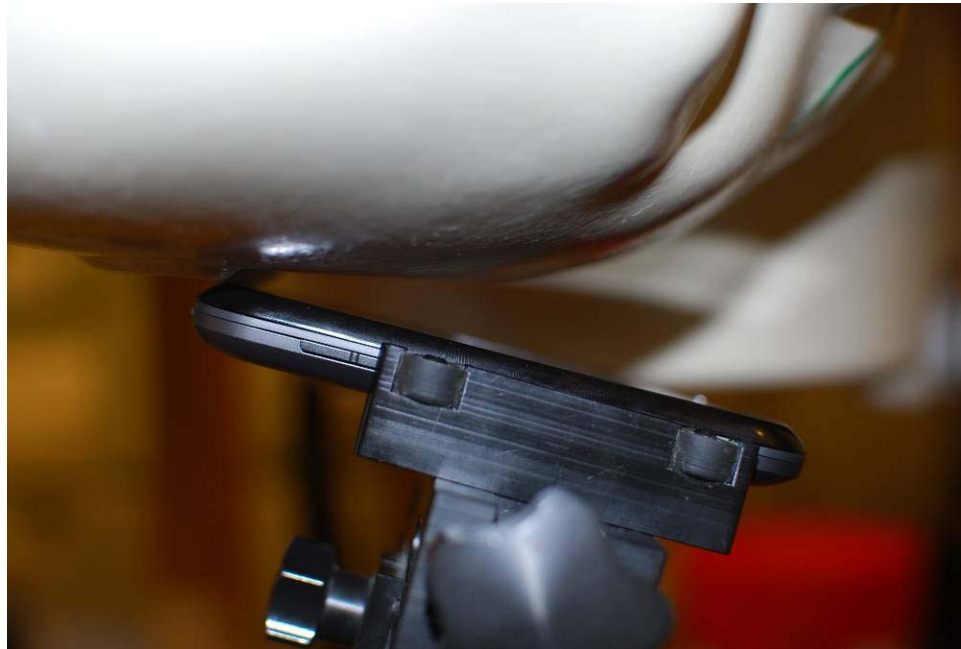
SAR Test Setup Photo 2 – Right Tilt
