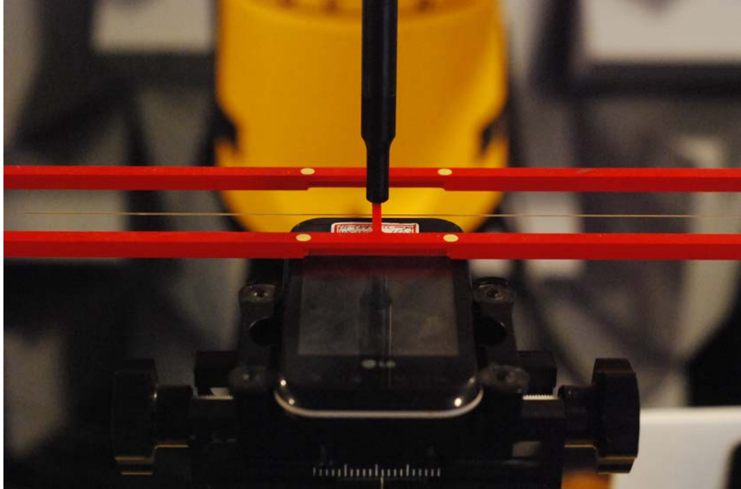
Figure 17-1 Ear Reference Point HAC Phantom Alignment
