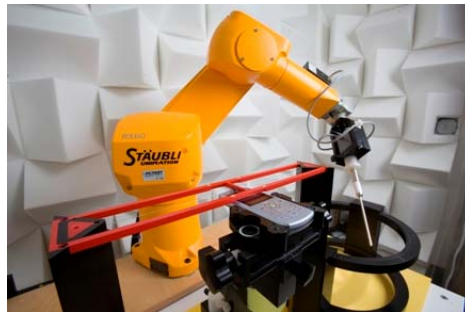
Figure 5-5 SPEAG Robotic System
