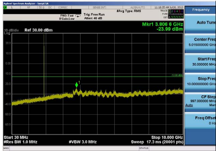
Plot 6-20. Conducted Spurious Plot (PCS GSM Mode – Ch. 810)
