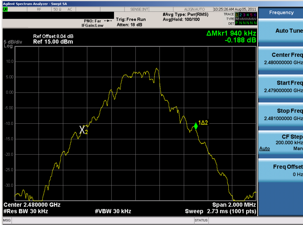
Plot 6-3. 20dB Bandwidth Plot (Bluetooth, 1Mbps – Ch. 78)
