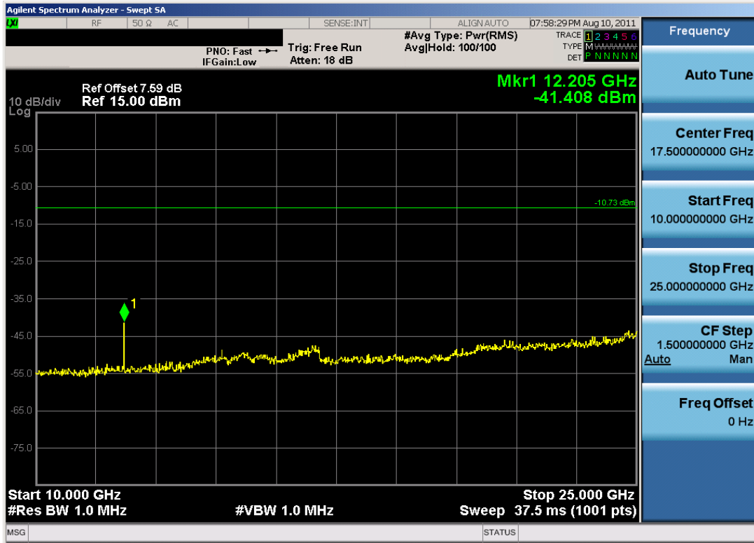
Plot 6-19. Conducted Spurious Plot (Bluetooth, 3Mbps – Ch. 39)
