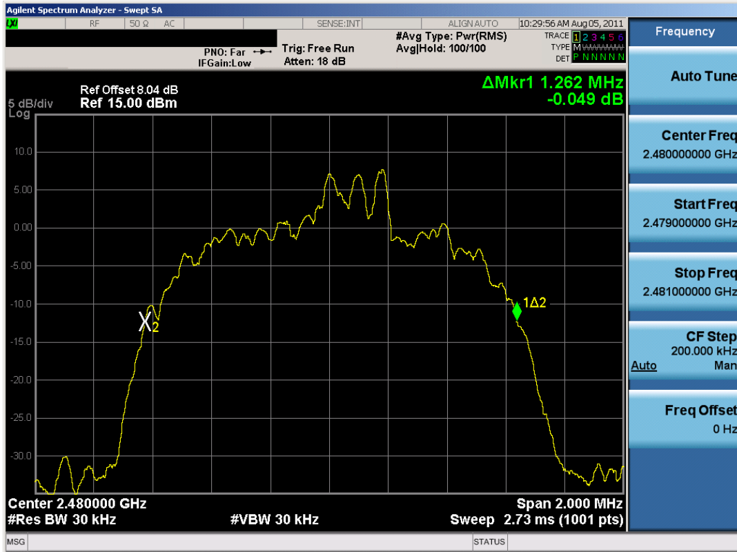
Plot 6-9. 20dB Bandwidth Plot (Bluetooth, 3Mbps – Ch. 78)
