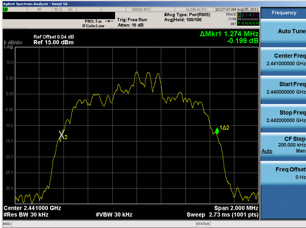
Plot 6-5. 20dB Bandwidth Plot (Bluetooth, 2Mbps – Ch. 39)
