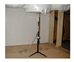
Figure 9.1 Dipole Validation Test Setup
