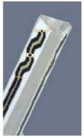
Figure 3.3 Probe Thick-Film Technique
