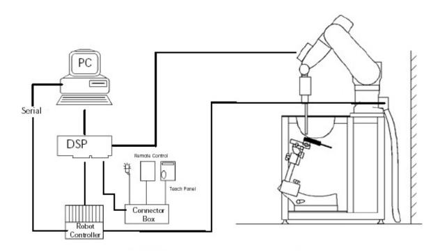
Figure 3.1 SAR Measurement System Setup
