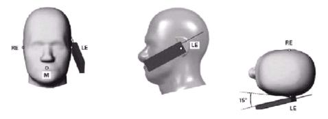
Figure 6.6 Front, Side and Top View of Ear/15°Position
