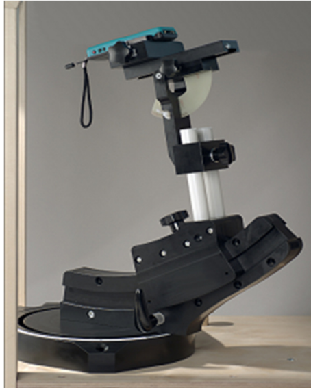
F-2. Device Holder for Transmitters
