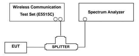
(Configuration of conducted Emission measurement)
