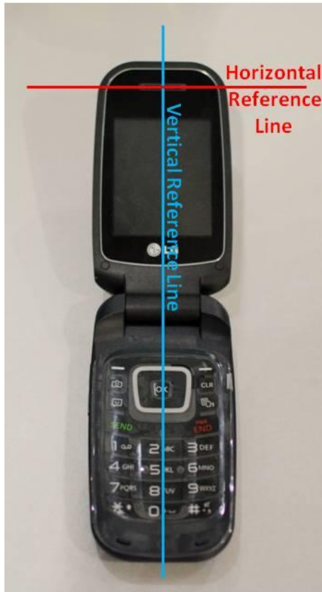
SAR Test Setup Photo 6 – Horizontal and Vertical Reference Lines
