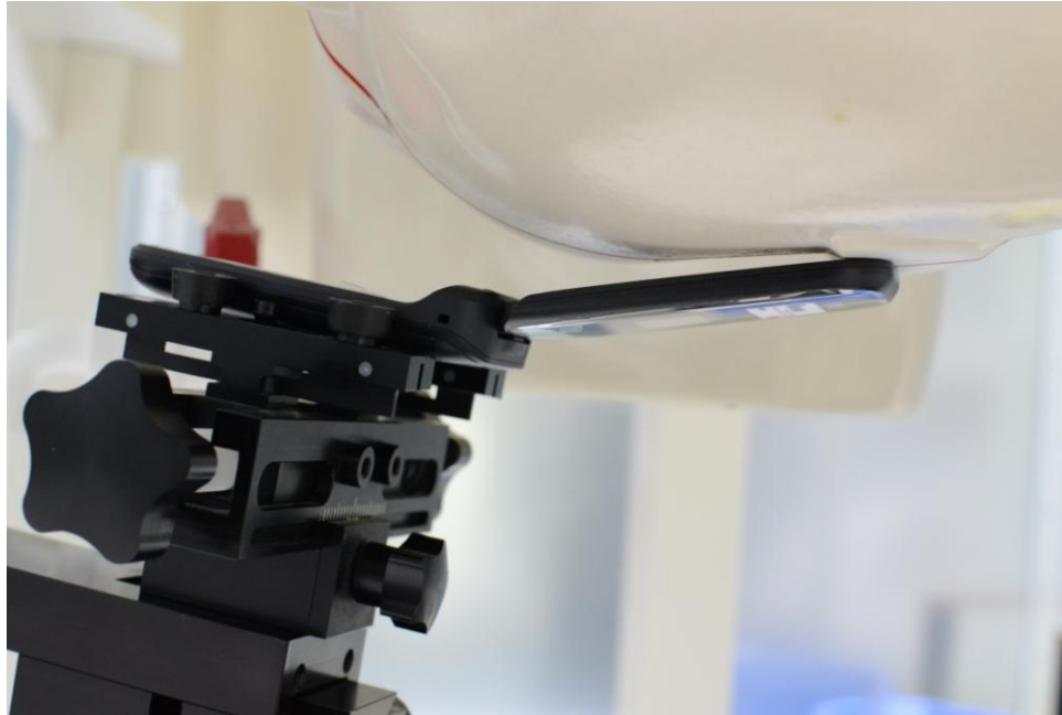
SAR Test Setup Photo 4 – Left Tilt
