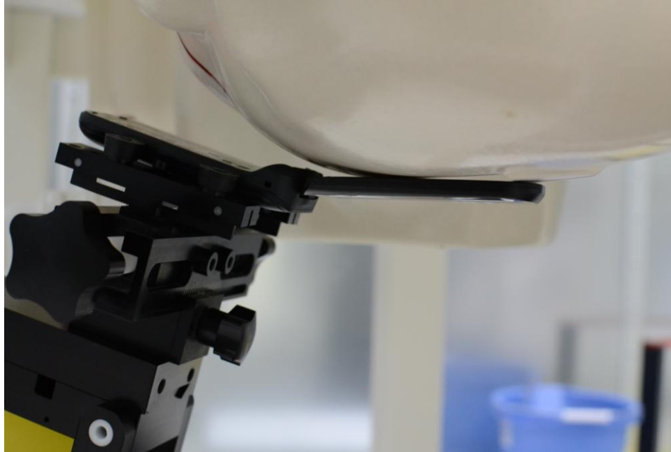
SAR Test Setup Photo 3 – Left Cheek
