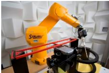
Figure 5-5 SPEAG Robotic System
