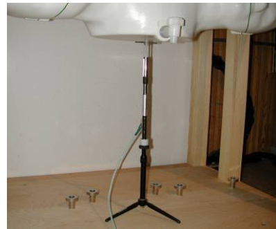
Figure 10-2 System Verification Setup Photo
