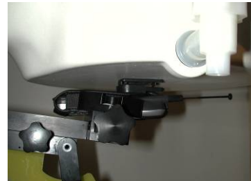
Figure 6-4 Body SAR Sample Photo (Not Actual EUT)
