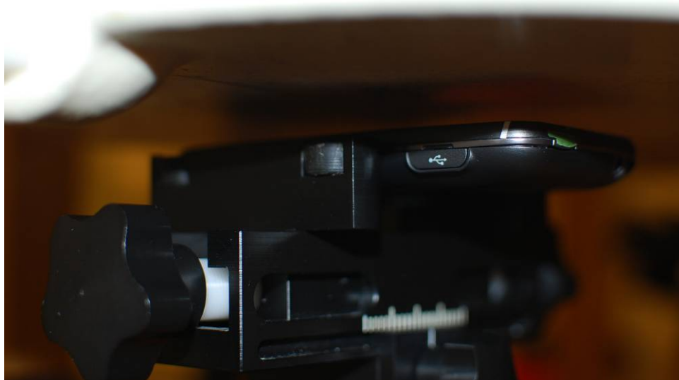
SAR Test Setup Photo 6 – Body Front at 1.0 cm
