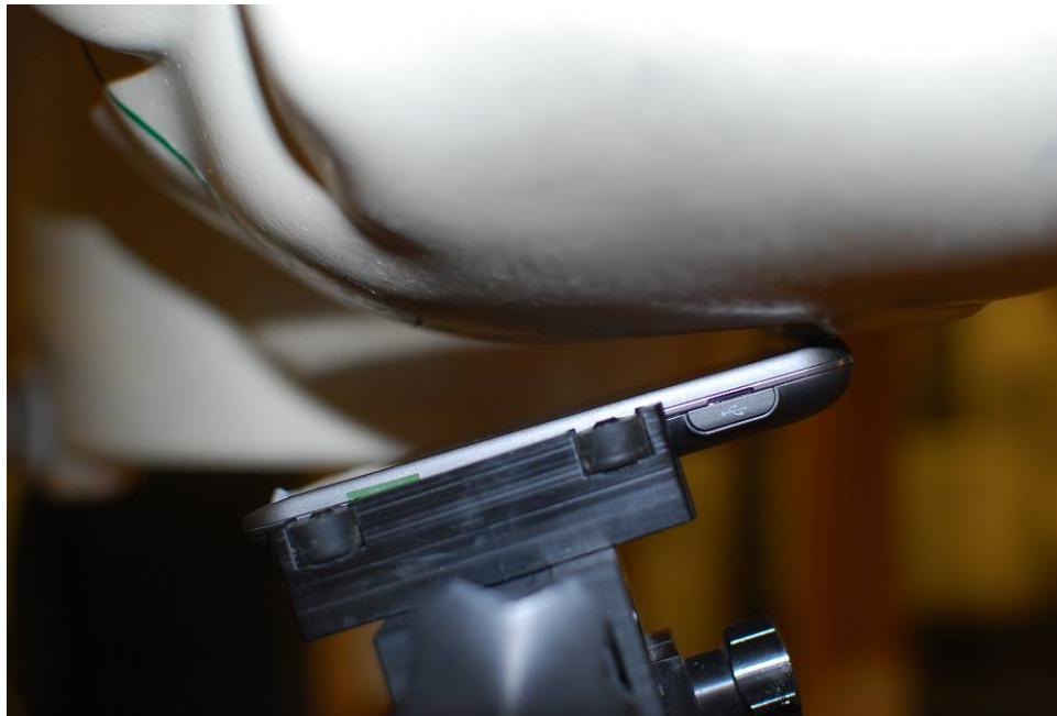
SAR Test Setup Photo 4 – Left Tilt
