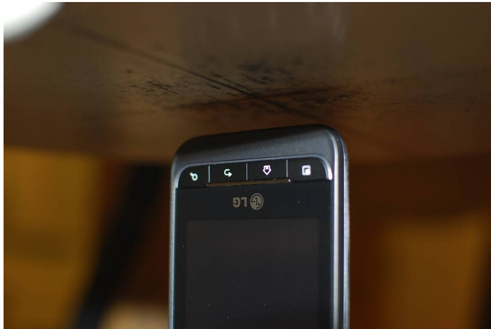
SAR Test Setup Photo 8 – Body Bottom at 1.0 cm
