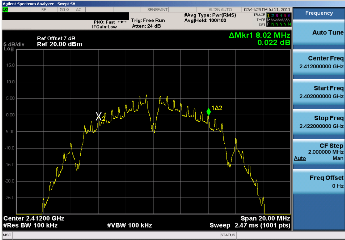
Plot 6-1. 6dB Bandwidth Plot (802.11b – Ch. 1)
