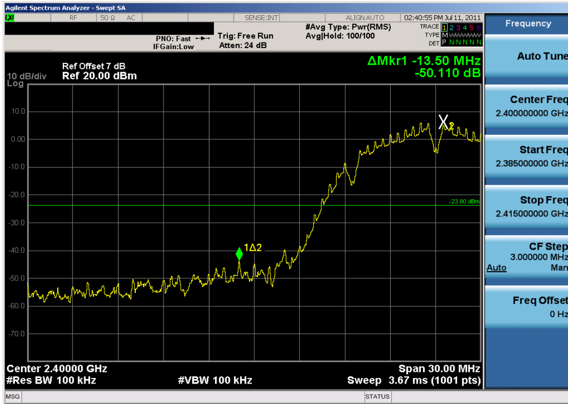
Plot 6-19. Band Edge Plot (802.11b – Ch. 1)
