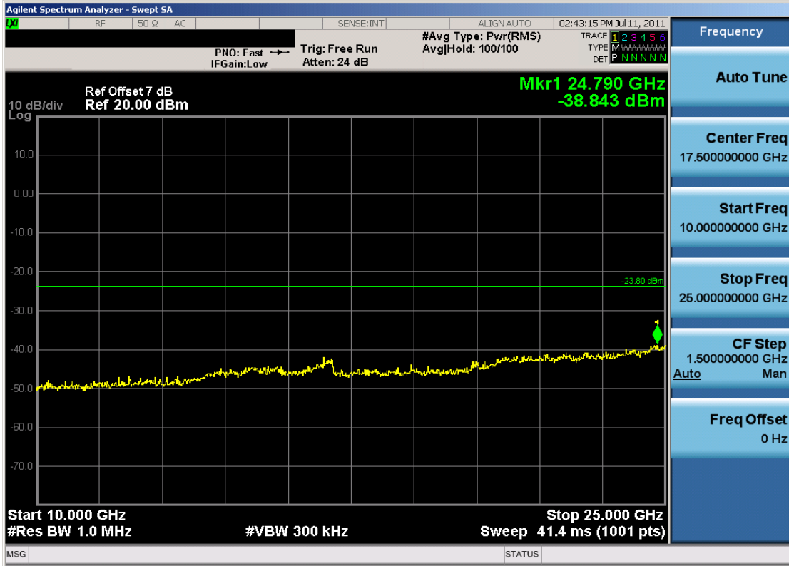
Plot 6-26. Conducted Spurious Plot (802.11b – Ch. 1)
