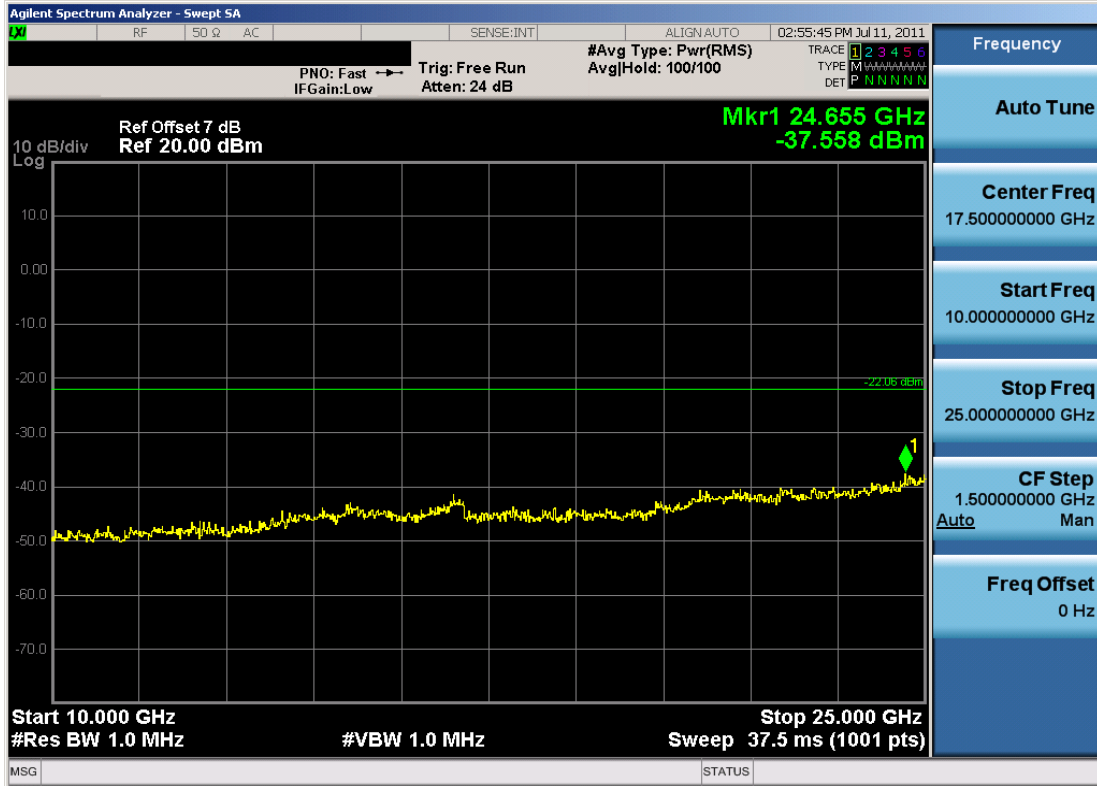
Plot 6-30. Conducted Spurious Plot (802.11b – Ch. 11)
