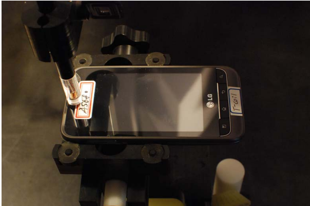
Figure 13-1 Test Setup for Wireless Device
