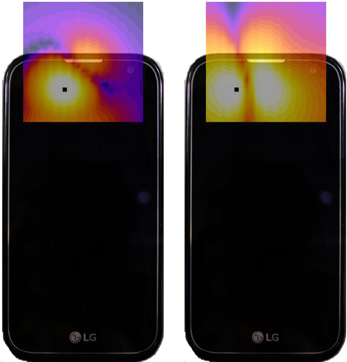
Figure 13-3 T-Coil Scan Overlay Magnetic Field Distributions
