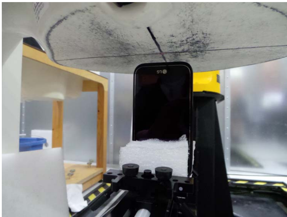
SAR Test Setup Photo 8: Bottom Edge at 10 mm
