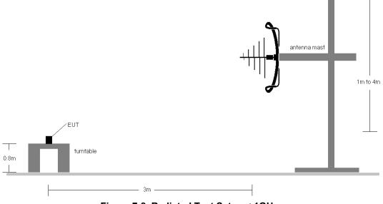
Figure 7-8. Radiated Test Setup < 1GHz
