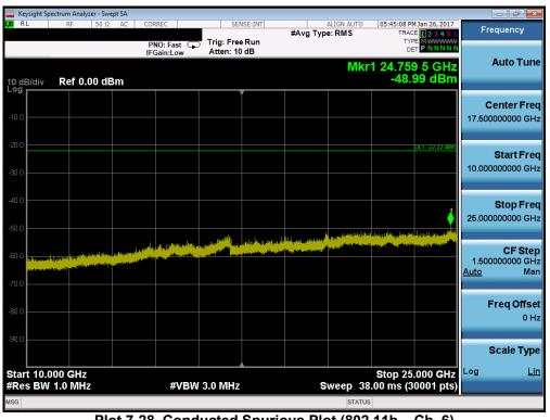
Plot 7-28. Conducted Spurious Plot (802.11b - Ch. 6)
