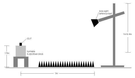
Figure 7-6. Test Instrument & Measurement Setup
