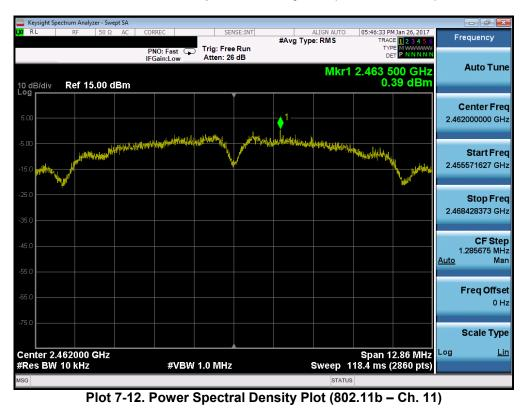
PCTEST Approved by: FCC Pt. 15.247 802.11b/g/n MEASUREMENT REPORT 🕒 LG FCC ID: ZNFAS110 (CERTIFICATION) **Quality Manager** Test Report S/N: Test Dates: EUT Type: Page 23 of 59 1M1701230039-04.ZNF 1/23 - 2/14/2017 Portable Handset © 2017 PCTEST Engineering Laboratory, Inc. V 6 2
