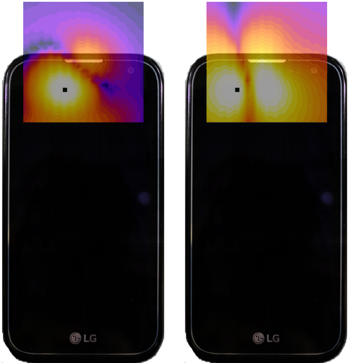
Figure 13-3 T-Coil Scan Overlay Magnetic Field Distributions
