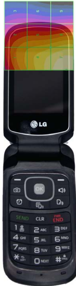
Figure 17-5 H-Field WD Scan overlay
