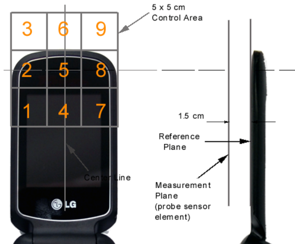
Figure 17-3 5x5 Scan grid above WD
