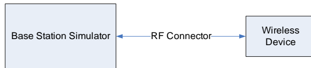
Figure 8-1 Power Measurement Setup
