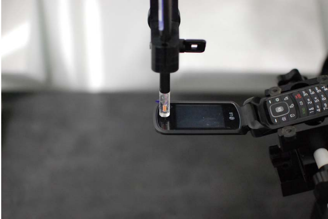
Figure 13-1 Test Setup for Wireless Device
