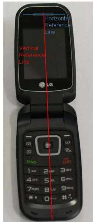
SAR Test Photo 6- Horizontal & Vertical Reference Lines
