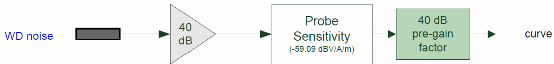
Figure 6-2 Audio Band Magnetic Curve Measurement Block Diagram
