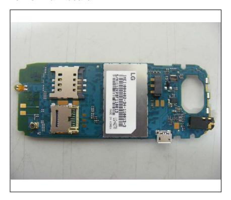
Bottom view of main board (Removing Shield)
