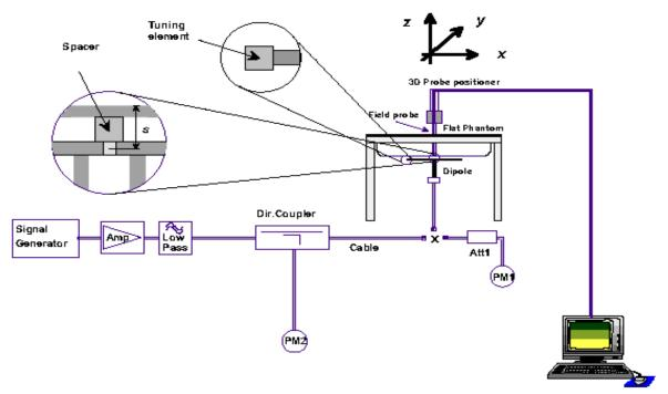
Fig b. System verification Setup Diagram
