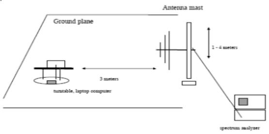
Test Procedures: Radiated emissions were measured according to ANSI C63.10.
