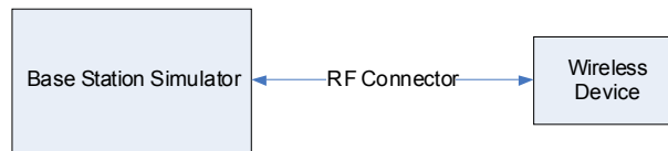
Figure 8-2 Power Measurement Setup
