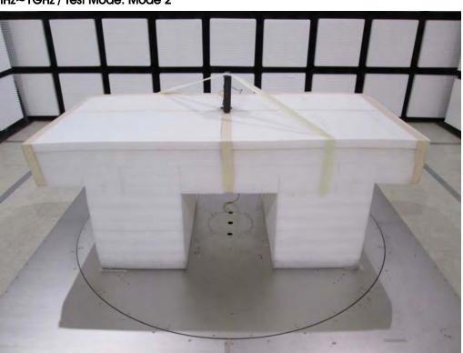
Test Configuration: 30MHz~1GHz / Test Mode: Mode 2
