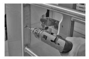
2. Fasten the antenna box to the side part of the feeding box using the screws enclosed so that the flat side faces the rear (see figure).
