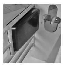
3. Feed the antenna cable through the cable opening that you drilled before.
