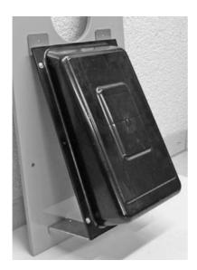
5. Drill a hole into the front plate directly beneath the antenna box and feed the antenna cable through it.
